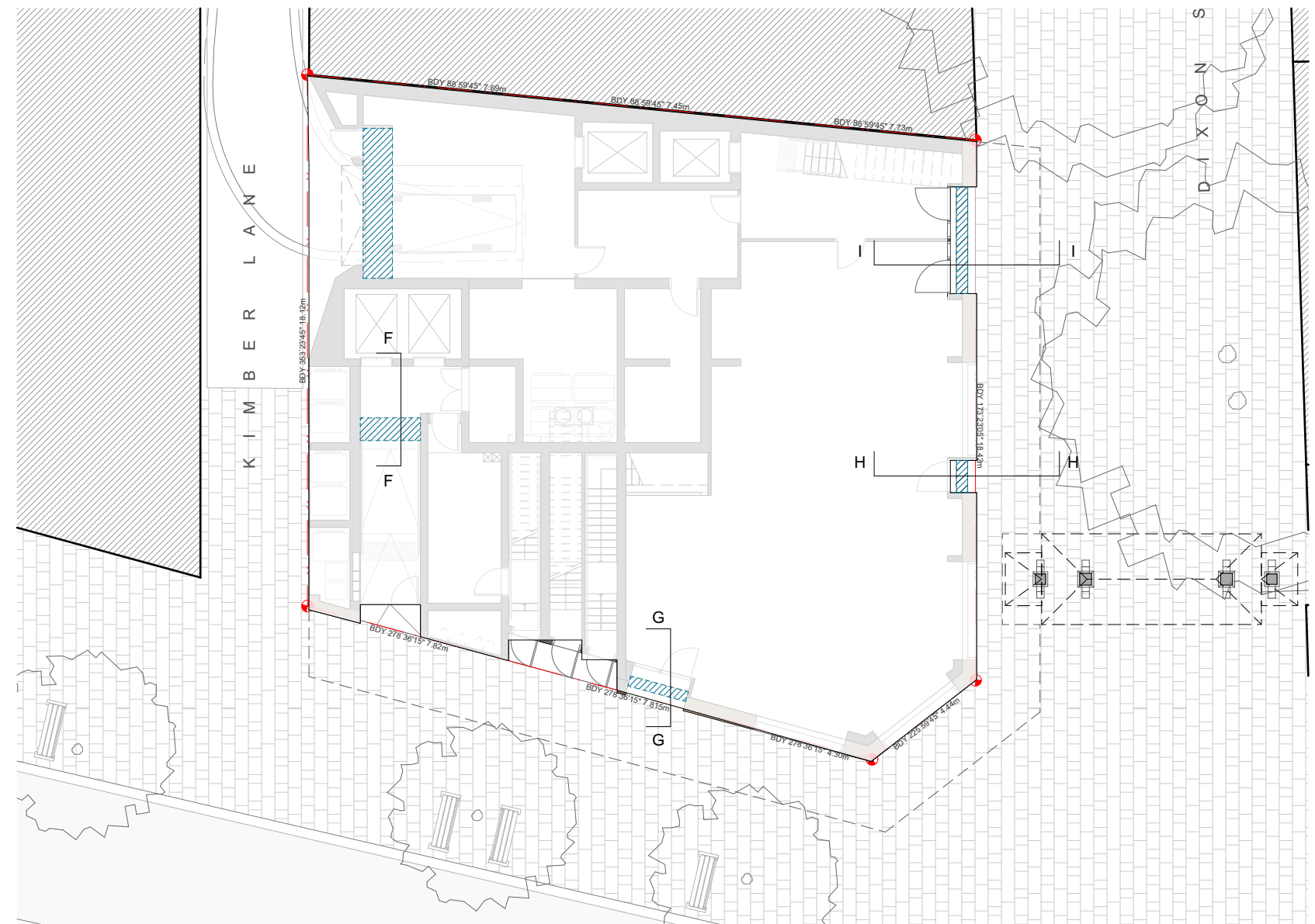
5 FLOOD GATE DIAGRAM - GROUND FLOOR PLAN 1:200
