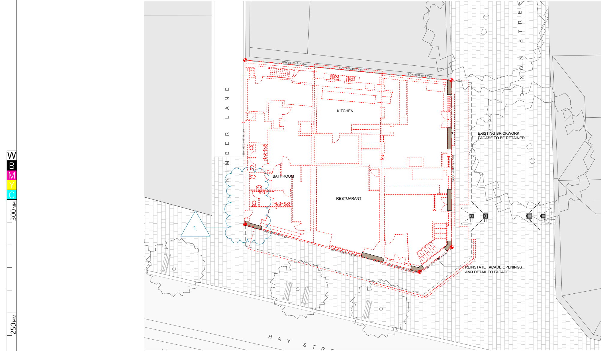
GROUND FLOOR DEMOLITION PLAN 1:250
